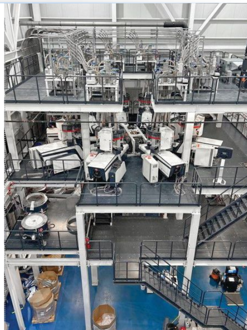
Plastilene's investment in W&H's water-quenched Aquarex film extrusion line has enabled it to penetrate high-end barrier packaging markets for meat and poultry. Source: Plastilene
