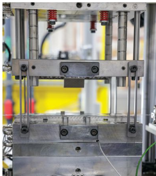
In addition to the press, Sodick provided tooling for the vertical overmolding cell. Source: Sodick
