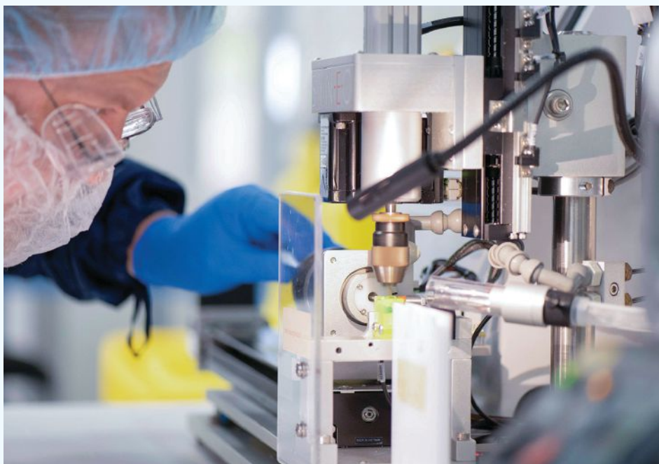
A technician closely monitors an automated bonding system during catheter assembly, ensuring precision alignment and secure connections at micron-level accuracy.
