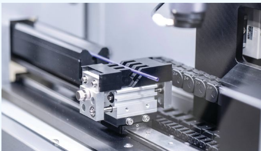
An automated precision testing system grips and inspects a catheter tube segment, showcasing advanced quality control technology used to ensure dimensional accuracy, lumen integrity and structural performance in high-spec medical tubing.
