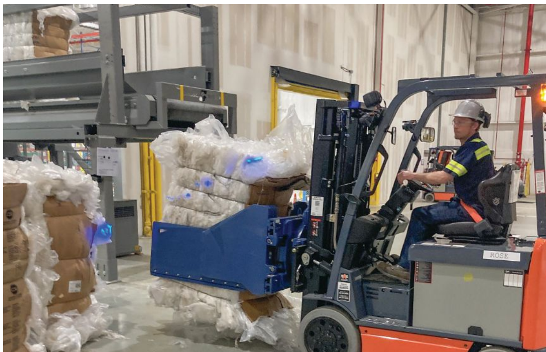
A bale is loaded onto the feed conveyor for the bale opening machine in Connersville, a rare hands-on step in an operation that is largely automatic.
