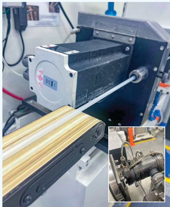
Two views of a precision multilumen extrusion line in action, showcasing the extrusion die (inset) and downstream puller mechanism guiding ultrathin medical tubing during production.
