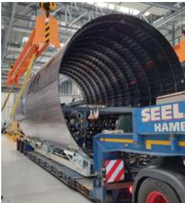
FIG. 6 The MFFD with welded assembly completed. Source | Aittip
