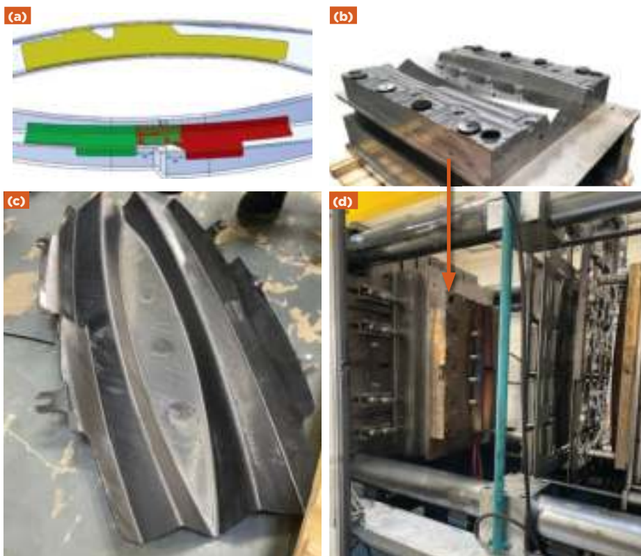
FIG. 5 (a) Three coupler parts were made in one set of matched molds that featured (b) springs in the center to keep tension on the laminates during stamp forming. Preheated TPC sheets were placed into the mold set in (c) an injection molding press where they were stamp formed into (d) double-curved parts that were then trimmed and ready for welding to frames. Source | Aitiip
