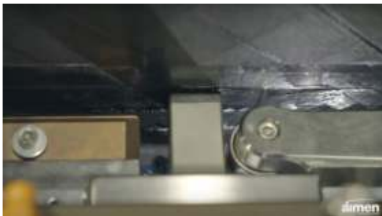
FIG. 3 The ultrasonic welding head (center) with roller on right and cooling/consolidation block on left. Source | AIMEN
