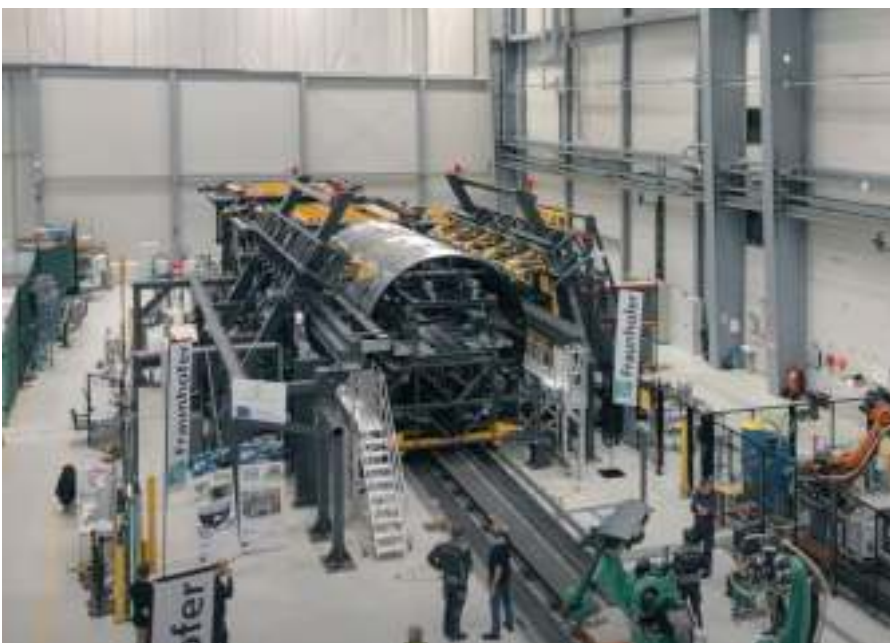
FIG. 1 The MFFD in the automated assembly facility developed in the MultiFAL project. Source | AIMEN
