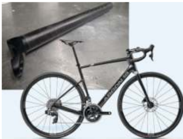
Canadian bike manufacturer Argon 18 currently makes road bikes based on thermoset composites, but sees a place for thermoplastics to grow in the future. This TPC seat post demonstrator showcased design and manufacturing possibilities. Source | CDCQ, LxSim and Argon 18
