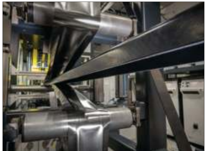
■ ATC’s continuous compression molding systems can produce larger structural parts such as ribs and bulkhead components.
