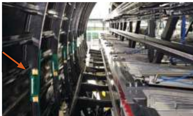
FIG. 4 Aitiip developed a tool that could be moved along a linear rail to position and then resistance weld TPC couplers (green parts at left of top photo) onto upper and lower fuselage frames, creating integrated structures across the RH and LH fuselage joins. The tool was also reversible, capable of being disassembled and mounted on the other side of the fuselage, to weld both RH and LH frames (below). Source | Aitiip
