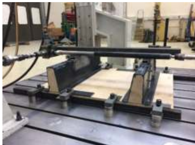
■ Interface validation test setup for composite-to-metal connections in the CFRP chassis. Load measurements in multiple directions ensure robust joint performance. Source | CarbonTT
