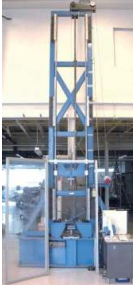
FIG. 2 University of Utah drop tower used for C-channel crush testing 2 .
