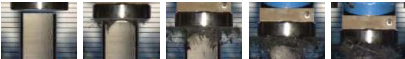
FIG. 3 Progressive crush behavior of composite C-channel specimen recorded using a high-speed video camera 2 .
