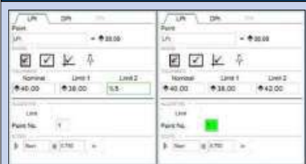
Figure 1 - testing software can aid in converting tolerance percentage to loads to prevent mathematical or transcription errors by the operator
