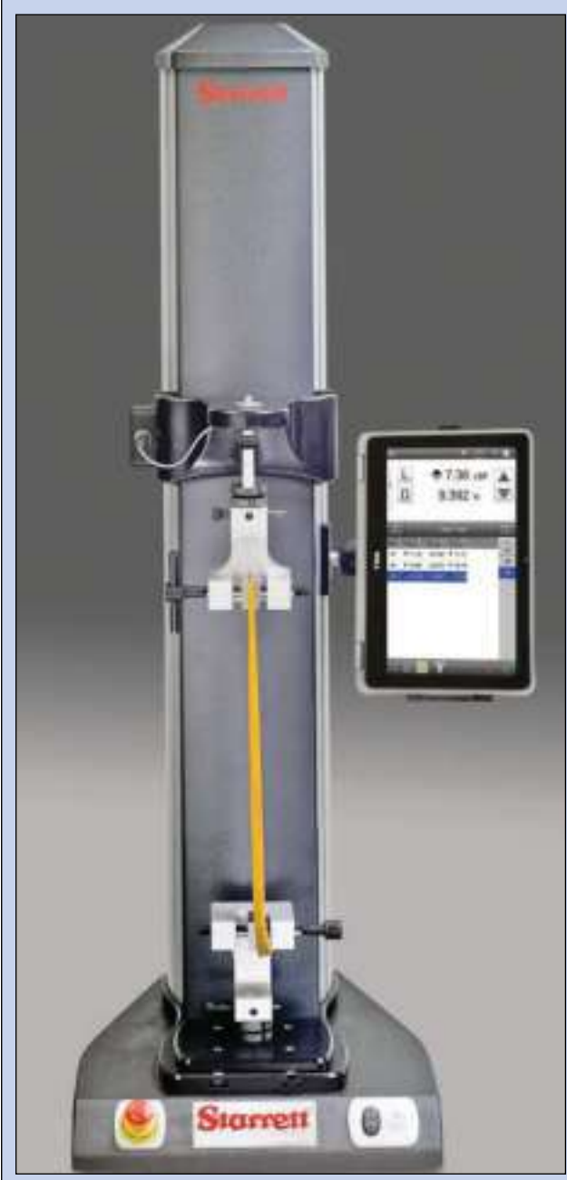
Figure 4 - Starrett FMS-1000-L2 250 pound capacity force measurement system running L2 software performing a tensile test on a rubber sample
