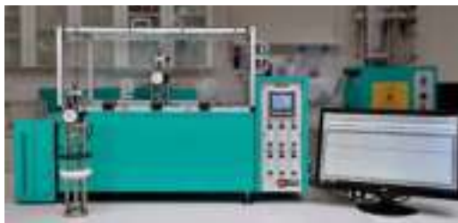
Stress relaxation test system for continuous testing of rubber in both tension and compression.
