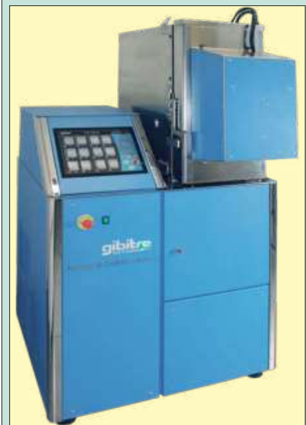
Figure 1 - DeMattia fatigue check AI camera
