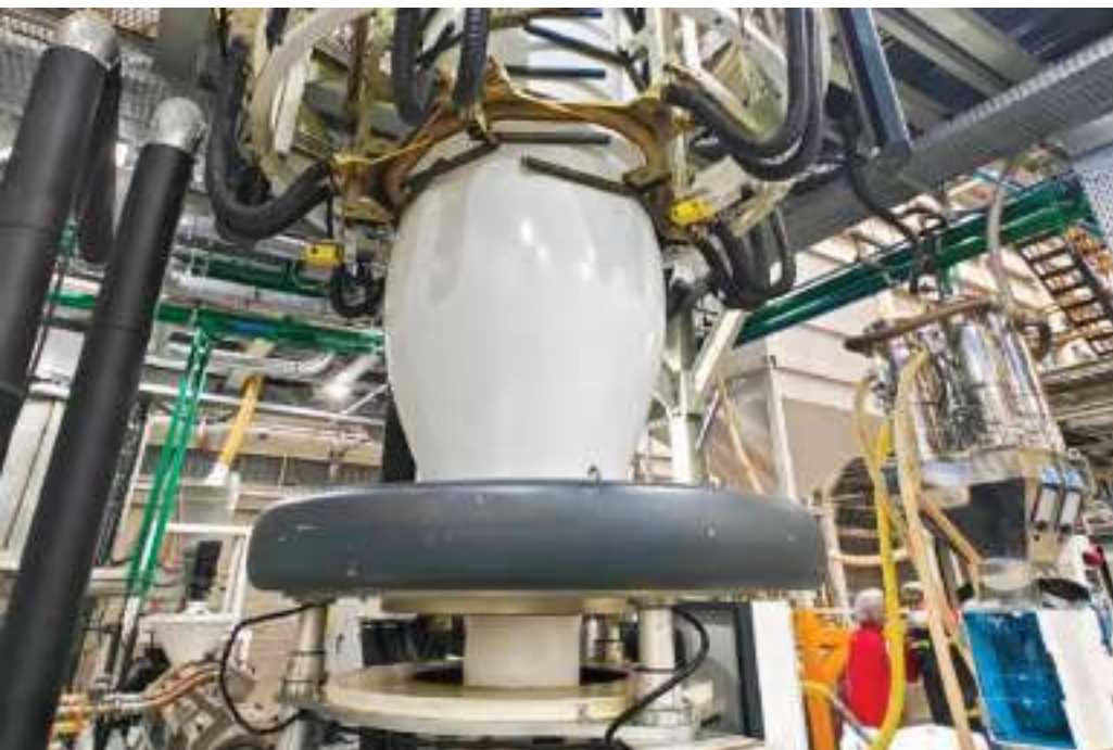
EVO Fusion system processes postindustrial recycled materials (PIR), enabling the recovery of production floor waste such as barrier films with printing and lamination.
