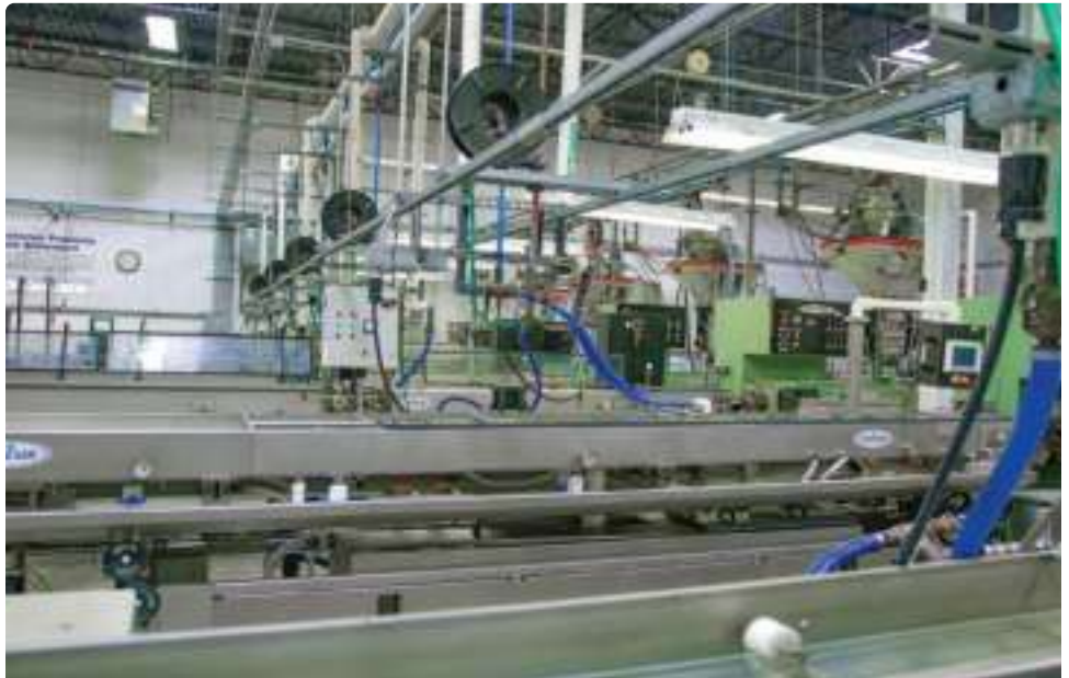
On each of its six extrusion lines, KEP relies on downstream cooling/sizing, pulling and cutting technology from Conair.
