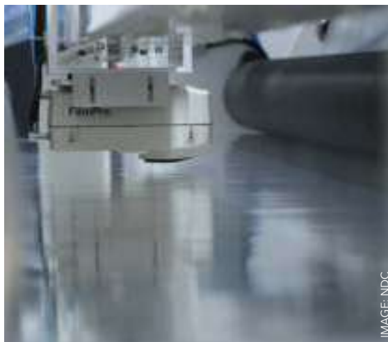
Left: NDC says FilmPro gauge offers accurate thickness measurement of film and sheet
