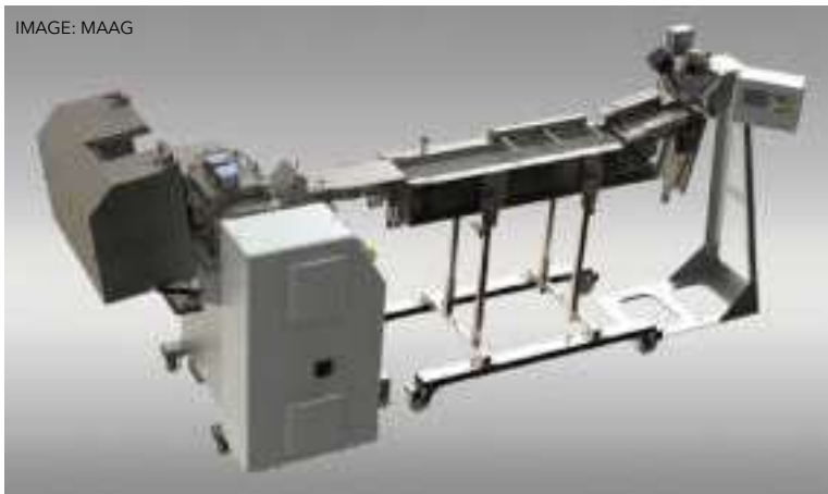
Above: Maag developed its semi-automatic single-belt EBG pelletising system for compounding sensitive, highly filled, or brittle products
