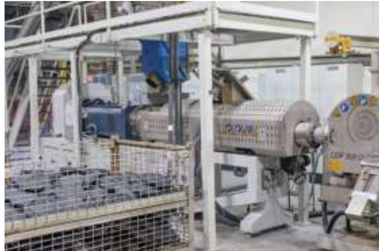
MAS extruder with magnetic separator system and melt filter. At left are collected patties of scrap from the melt filter, which will be reprocessed to extract usable polypropylene.
