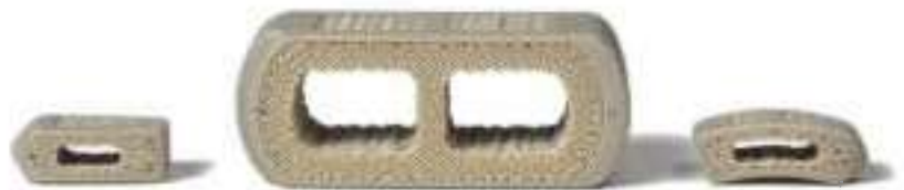
3D printing enables each layer to be put in compression as it is deposited through FSD, and also makes possible novel porous structures that support osseointegration.
