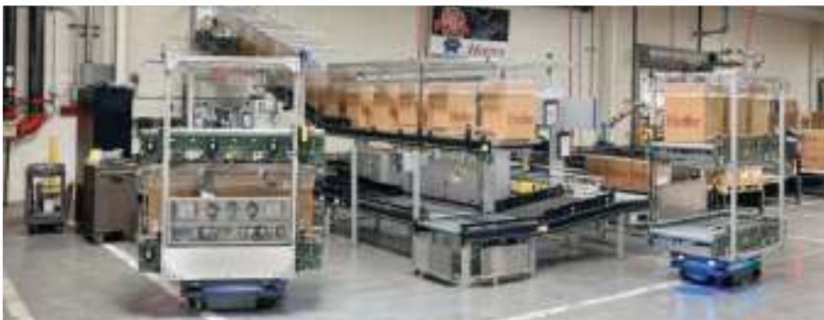
Hoffer Plastics deploys custom-designed autonomous mobile robots (AMRs) to ferry finished goods around its facility. Source (all images): Hoffer Plastics
