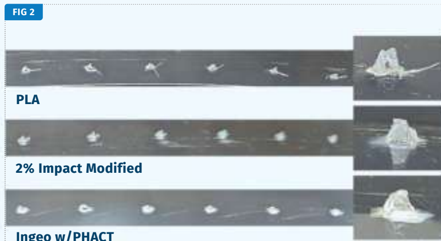
The Ingeo PLA/PHACT aPHA formulation exhibited a noticeable reduction in rail chipping due to its greater durability.
