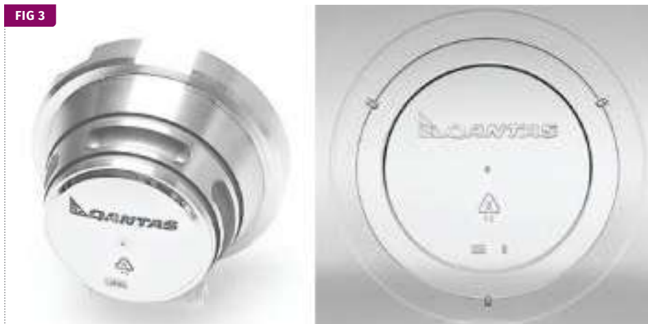
Gate pad engraving in steel and in the bottom of a molded container.
