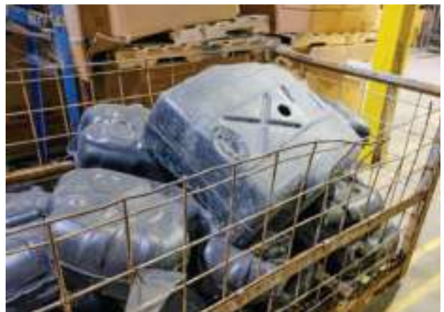
These gas tanks, composed mainly of HDPE, will be recycled for sale into a variety of applications.
