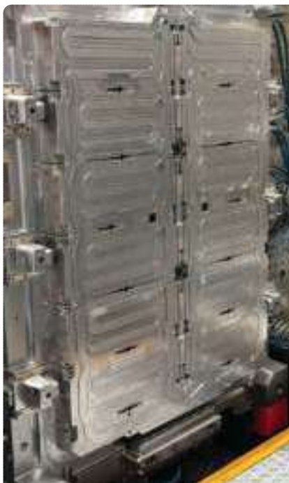
Siebenwurst built the molds for the battery tray (pictured) and cover. Source: Siebenwurst
