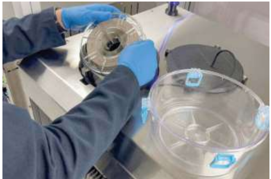
The PEEK filament undergoes a drying step before it is loaded into the 3D printers to produce implants.
