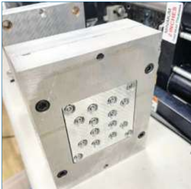
An aluminum mold made with ejector pins using a desktop Swiss CNC machine.
