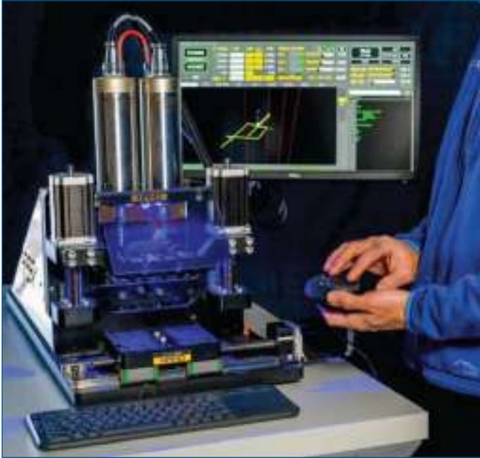
A precise, rigid desktop CNC Swiss lathe can machine metals and plastics.
