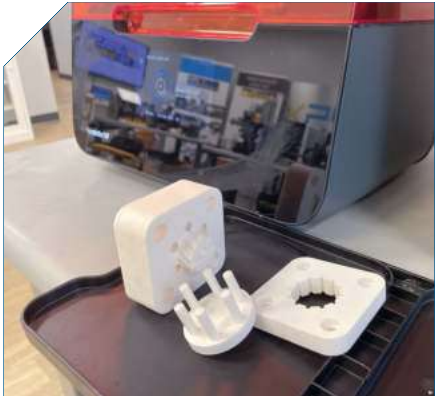
A mold produced on a desktop resin 3D printer. Source (All images) | APSX
