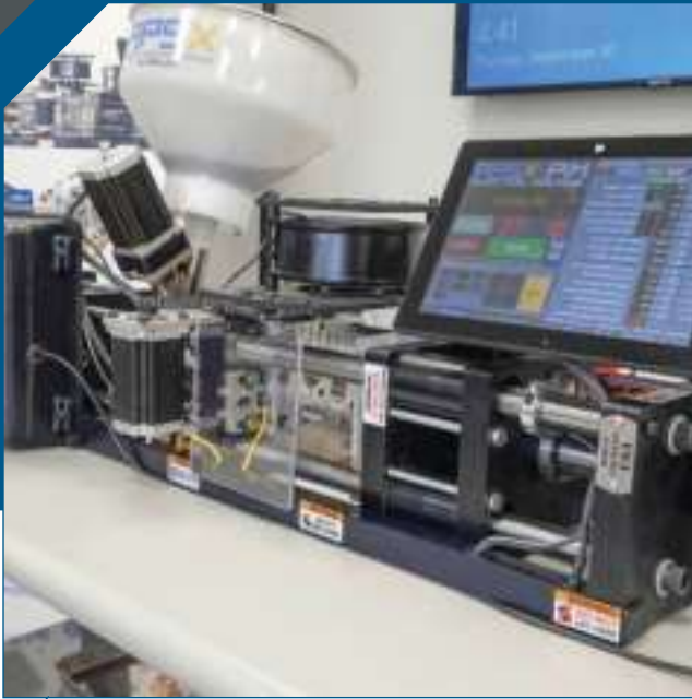
An automatic desktop plastic injection molding machine can make injection molding affordable and easy, including this heavy-duty machine for continuous or single-cycle plastic part production.
