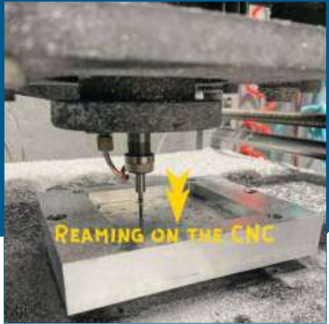
A highly precise, rigid, portable desktop CNC milling machine machines a mold. This machine can mill aluminum, steel, bronze, brass, delrin wood and plastics with high precision.
