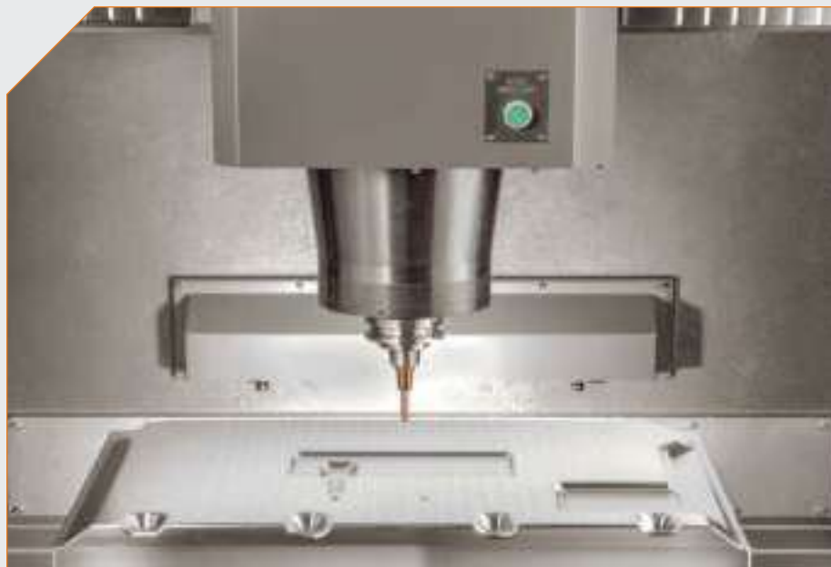
This large-capacity VMC can accommodate up to a 5,500-pound table load with 17 inches between columns. Smaller and mid-range machines are available.
