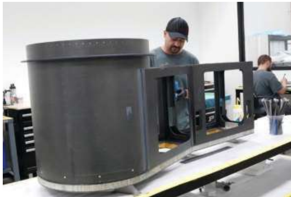
■ RWC technicians perform precision assembly for a large aperture telescope structure delivered to EOI Space.
