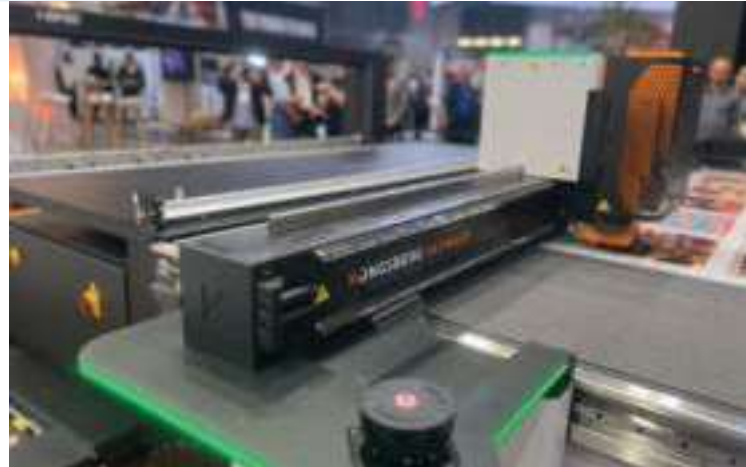
■ A lightweight and high-stiffness carbon fiber-reinforced polymer (CFRP) gantry beam enables the Ultimate's high-speed precision cutting. Source | CompoTech
