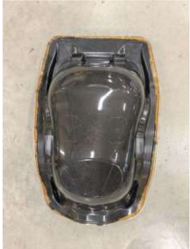
■ A side view of the F2 seat (above), and bottom-up view after being removed from the resin transfer molding (RTM) machine ahead of the belt holes being cut (right). Source | Faber
