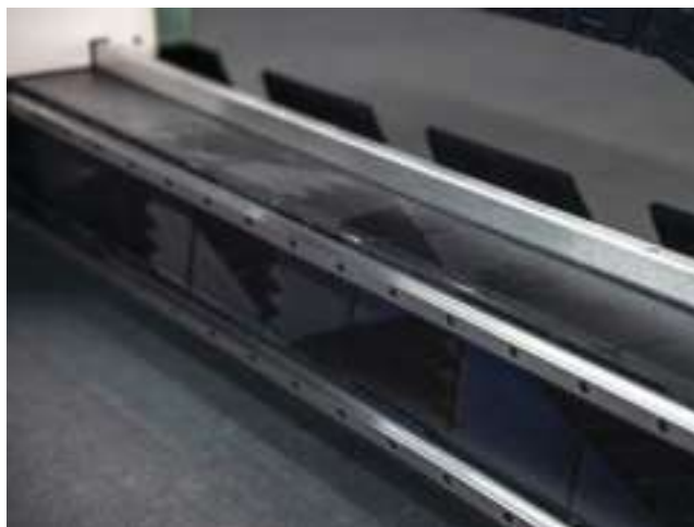
■ CFRP beam shows aluminum rails affixed by bolts into holes machined through carbon fiber side strips, then bonded to the beam into the aluminum rod inserts. Source | CompoTech, Kongsberg PCS
