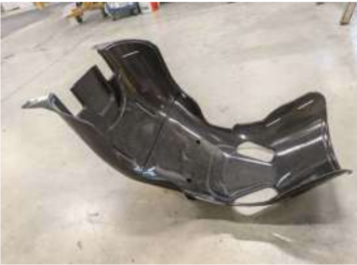
■ A side view of the F2 seat (above), and bottom-up view after being removed from the resin transfer molding (RTM) machine ahead of the belt holes being cut (right). Source | Faber
