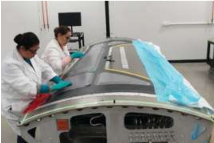
■ RWC technicians perform prepreg ply placement using a laser projected template.
