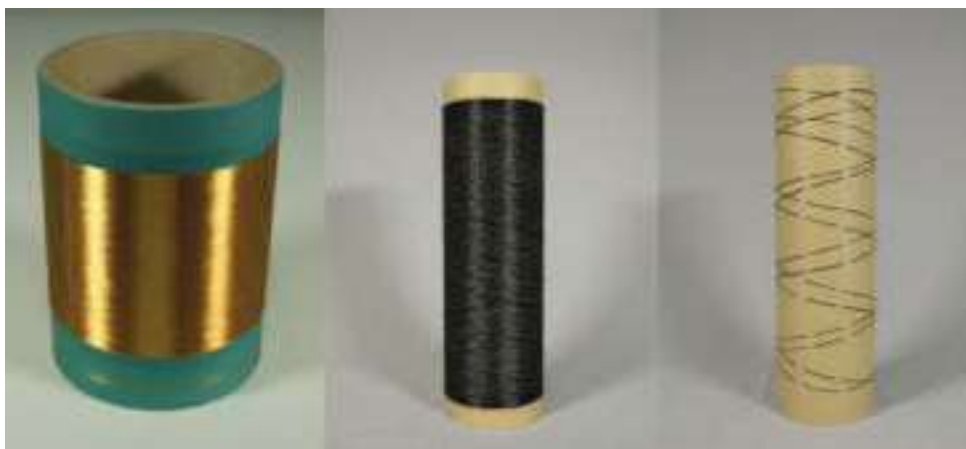
Water-spun lignin precursor fibers, stabilized and carbonized continuous filaments. Source | DITF
