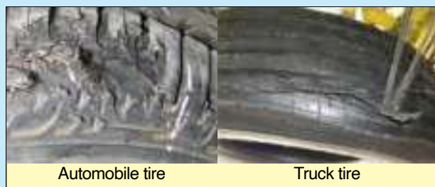
Figure 14 - belt edge separations in an automobile tire and truck tire
