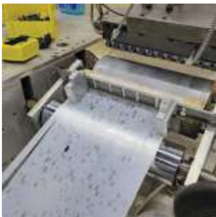
Here, undried nylon was processed on the MH. Bubbles were still created, left. After a single atmospheric vent was opened, exposing the extensive free surfaces, the film on the right was produced with no bubbles at the same rate.
