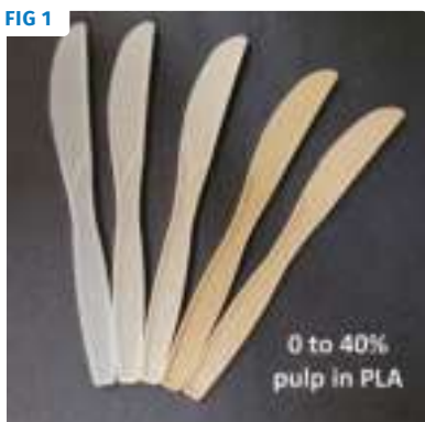
Applications for bioresin and wood pulp compounds include disposable cutlery. Source: FPIInnovations
