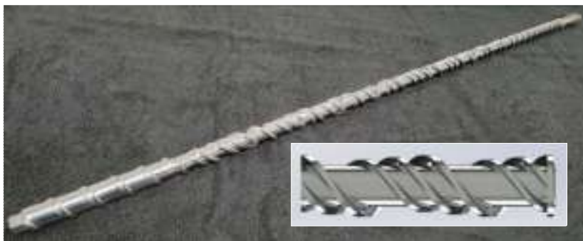
Randcastle’s Molecular Homogenizer is a 36:1 L/D screw with seven mixing sections. According to the inventor, it has been shown to enhance mixing and also improve material properties in some cases. Inset shows single mixing element. Source: Randcastle Extrusion
