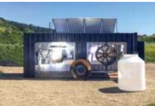
A solar rotational molding system with a sample rain catchment tank.
