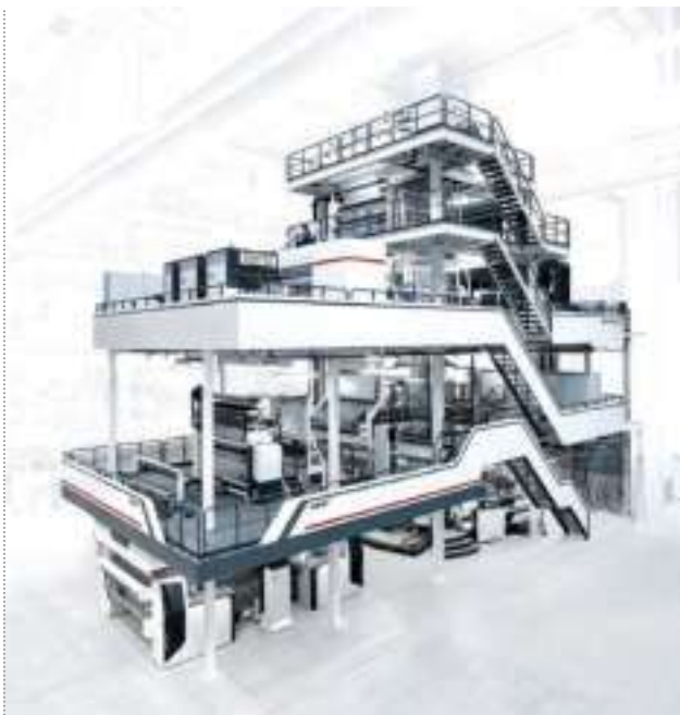
Malpack will be soon be adding its first two lines for blown film, including this Vares II 7-layer line for producing agricultural films. Source: W&H
