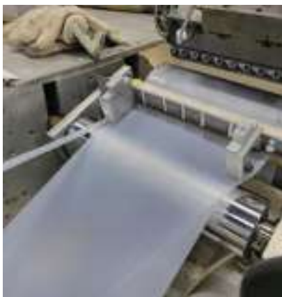
Here, undried nylon was processed on the MH. Bubbles were still created, left. After a single atmospheric vent was opened, exposing the extensive free surfaces, the film on the right was produced with no bubbles at the same rate.
