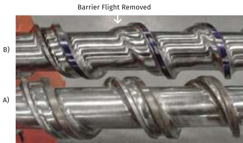
Photographs of barrier flight entries: (a) standard entry that had a rate restriction and (b) modified entry where the barrier flight was removed down to the root of the melt channel for the first 1.5 turns of the section.
