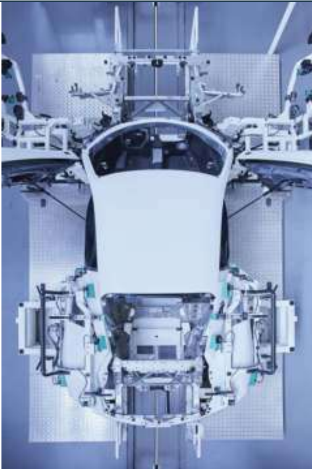
■ The Maserati MC20 features a body structure that highlights a composite central tub and roof structure, which are connected to two aluminum subframes at the front and rear. Source | Maserati
