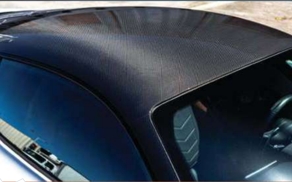
■ The carbon fiber composite roof of the Maserati MC20 is achieved using HP Composites' AirPower technology, a derivative of bladder-assisted compression molding (BACM). Source | Maserati
