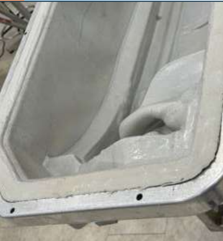
■ The custom counter mold for the construction of CFRP components using AirPower technology. Source | HP Composites
