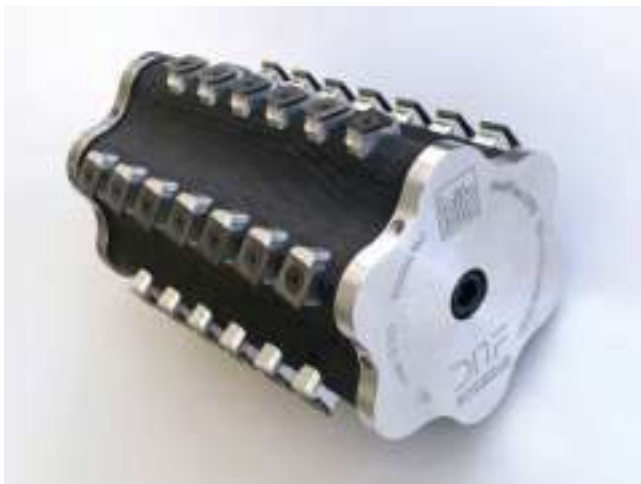
■ CFRP planing head reduces mass versus aluminum from 8 to 4 kilograms, enabling rotational speeds up to 18,000 rpm. Source (All Images) | DITF
