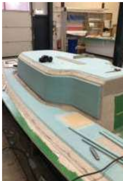
■ The entire exterior and inner structures for the Flax27 Daysailer are built with infused flax fiber composites with a bio-based epoxy and recycled PET foam core. Source | Greenboats
