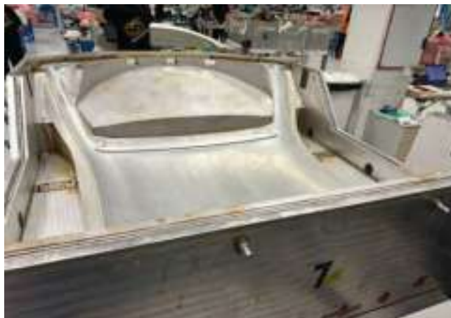
■ Vacuum line connections in the lower mold section of the Maserati MC20 roof mold enable the application of air pressure on the top and vacuum on the bottom of the flexible counter mold during manufacturing. Source | HP Composites
