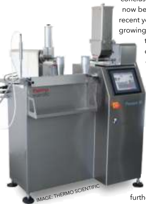
Above: Thermo Scientific's Process 16 twin-screw extruder can process as little as 5 kg to 10 kg of material
