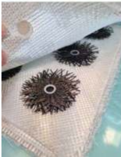
FIG. 1 The FiberJoints patch improves static strength and fatigue endurance of composite bolted joints. Source (All Images) | FiberJoints
