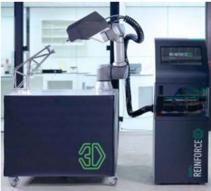
■ The CFIP machine includes a manual or robotic injection head programmed to inject specially treated fibers and liquid resin via designed fiber trajectories.
