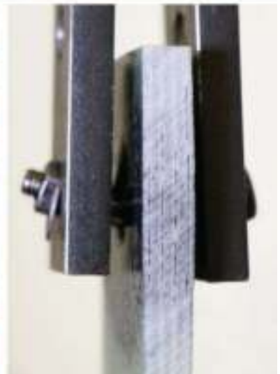
FIG. 1 The FiberJoints patch improves static strength and fatigue endurance of composite bolted joints. Source (All Images) | FiberJoints
