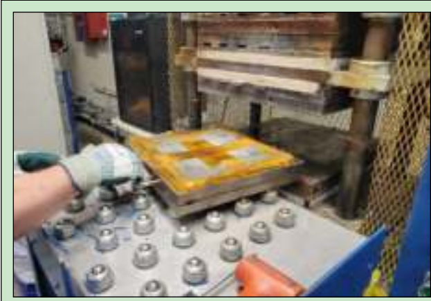
Figure 1 - compression molding can produce low volumes of USP Class VI silicone parts
