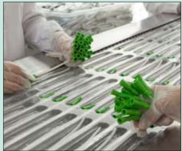
Figure 2 - connecting tubes to rigid fittings can be a labor intensive process in catheter production
