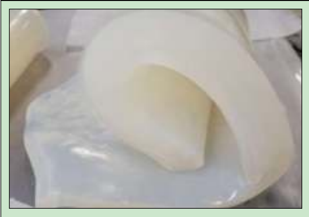
Figure 2 - calendaring is used to produce rolls of USP Class VI medical silicones
