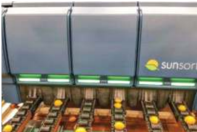
Custom-color ABS replaced sheet metal in the covers of these industrial sorters.
