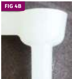
FIG 4B Restrictive and excessive sucker pin wells.
