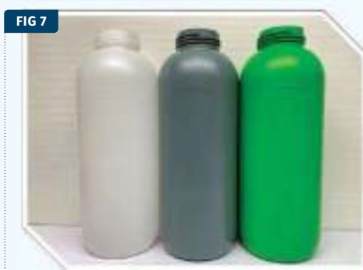
Topload strength comparison of virgin (left), monolayer PCR (center) and ReCo bottle with PCR (right).
