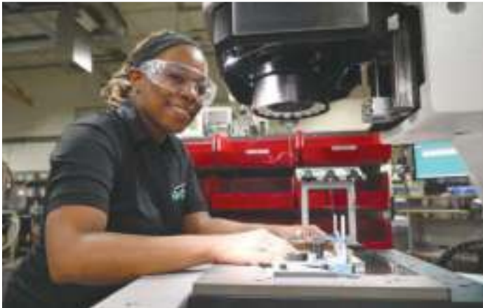
Nika Martin, CMM operator at Allegheny Performance Plastics, completes a quality check. Source: Allegheny Performance
