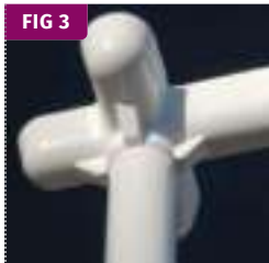
FIG 3 Gussets connecting a runner to a runner drop.
