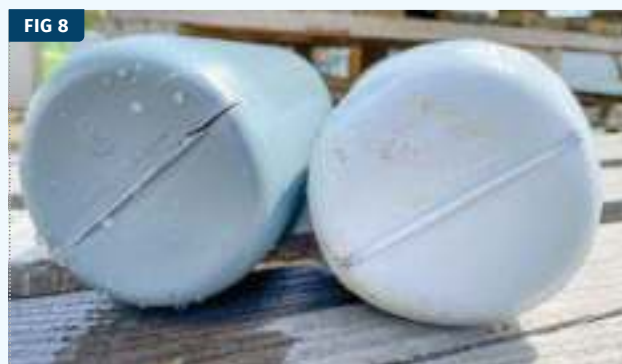
FIG 8 In drop tests, monolayer gray PCR bottle (left) split at the weld seam after two falls, while white ReCo bottle with PCR in main layer (right) survived five falls intact.
