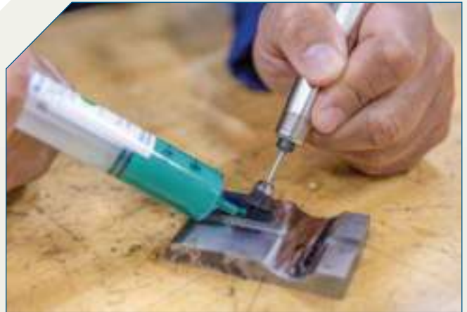
Diamond polishing compound options are available for hard or soft metals requiring different levels of precision. Source | Boride Engineered Abrasives
