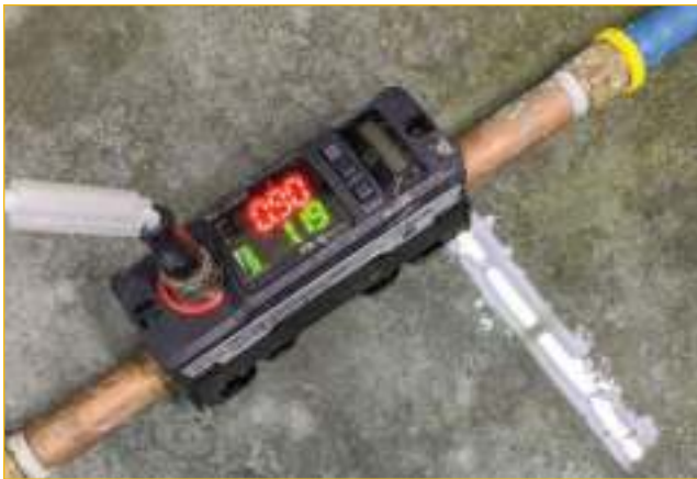
Flowmeter readings: Gallons per minute (GPM; flow rates) are displayed on the left, showing a 114% increase in flow. The bottom number is the user-set target GPM, adjustable to any desired value. Upon reaching the target, the light on the right turns green.
