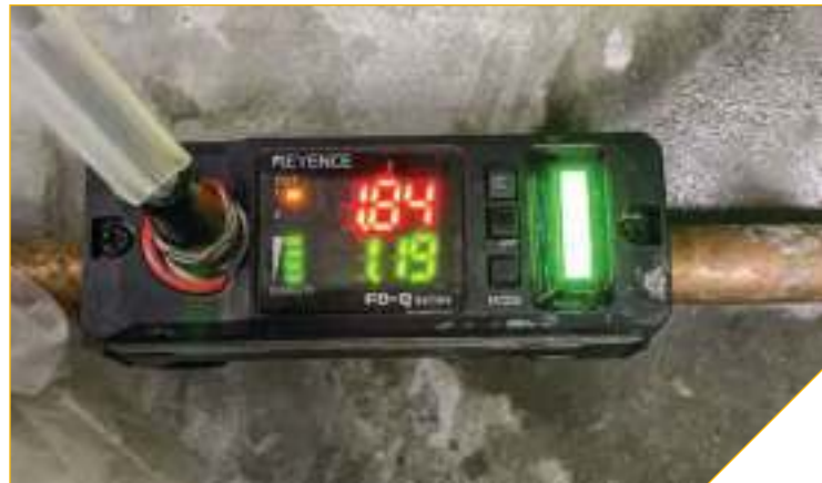
Flowmeter readings: Gallons per minute (GPM; flow rates) are displayed on the left, showing a 114% increase in flow. The bottom number is the user-set target GPM, adjustable to any desired value. Upon reaching the target, the light on the right turns green.
