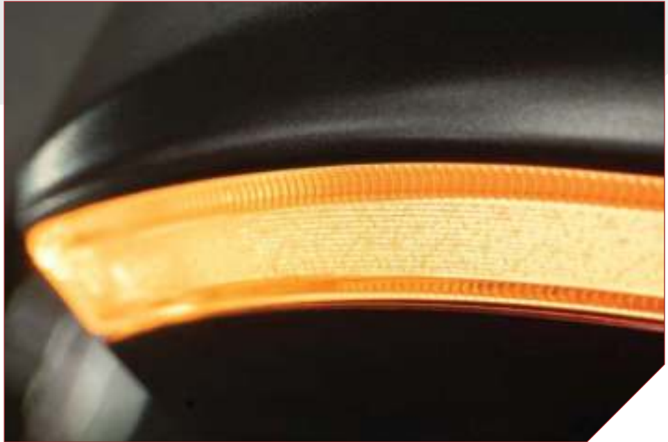
Ultra-fast femtosecond laser texturing enables mold builders to texture plastic and steel workpieces with sharp facet feature edges, eliminating the need for pre-textured test lenses.
