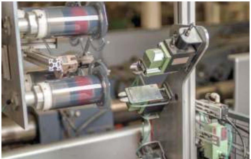
Custom injection molder Westec Plastics Corp. operates 23 injection presses (some of which are shown at top) and uses additively manufactured EOAT and fixtures produced on its own in-house printer or those of local service bureaus. Shown on the bottom is an EOAT that pulls molded parts for the consumer segment from a four-cavity injection tool and clips off the runners. Source | Westec Plastics Corp.
