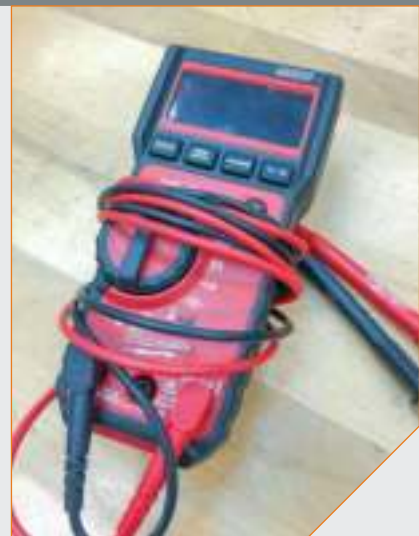
Ohmmeters test T/Cs and heaters for proper ohms and insulation resistance.
