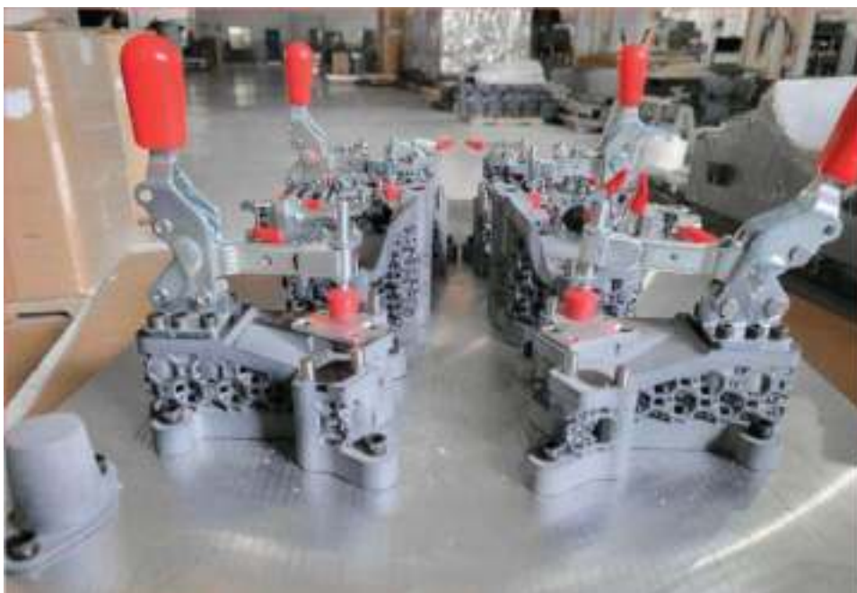
Taking advantage of additive manufacturing's ability to produce lattice structures, which not only reduce mass, material usage and cost and speed printing time, but also increase structural integrity, Linear AMS applies the technique to 3D print inspection fixtures like those shown above. The gray lattice material is PA12 produced on an MJF or SLS printer; the red handles/clamps and bolts are off-the-shelf purchased components; and the silver base plate is conventionally machined aluminum. Source | Linear AMS, a Shapeways Co.
