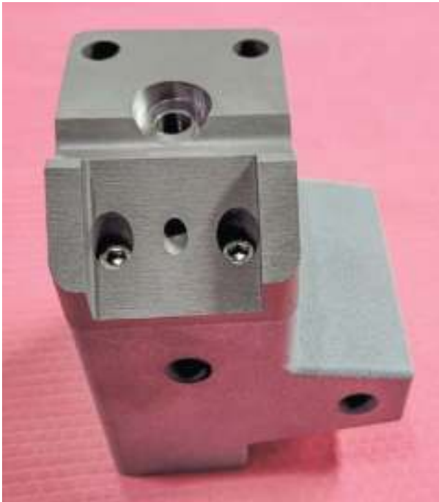
This inspection assembly fixture – a hybrid of metal and polymer additive technologies – features 3D printed maraging steel (top bronze components with bolts produced via direct metal laser sintering/solidification, or DMLS) and PA12 (lower gray component produced via MultiJet Fusion (MJF) or selective laser sintering (SLS)). Use of both additive technologies helps Linear AMS reduce mass, cost and print time while producing a usable assembly aid much faster than conventionally machined metal would allow. Source | Linear AMS, a Shapeways Co.
