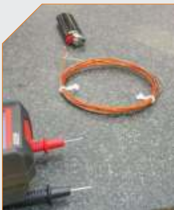
T/Cs are the feedback loop for the temperature of a manifold.
