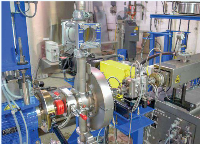
Twin-screw extruder furnished with a gear pump and an underwater pelletizing die.
