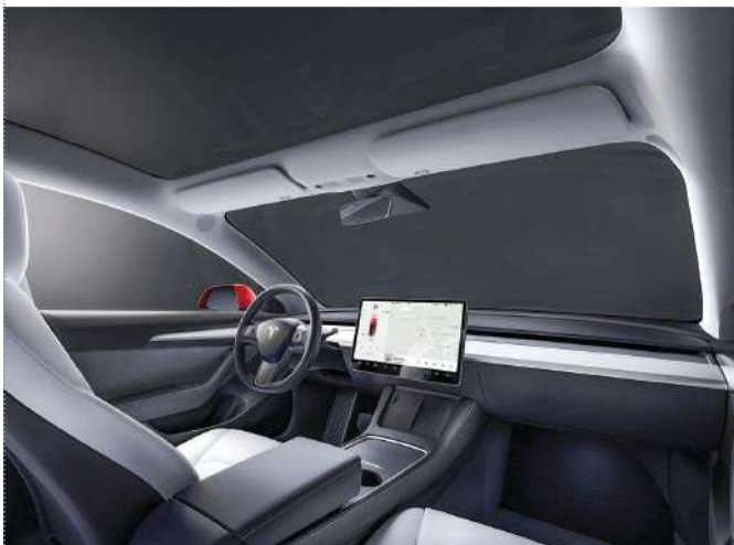
Tesla has had multiple effects on auto manufacturing, including in the interior, where the traditional knobs and buttons have been eliminated, as in this Model 3. Source: Tesla
