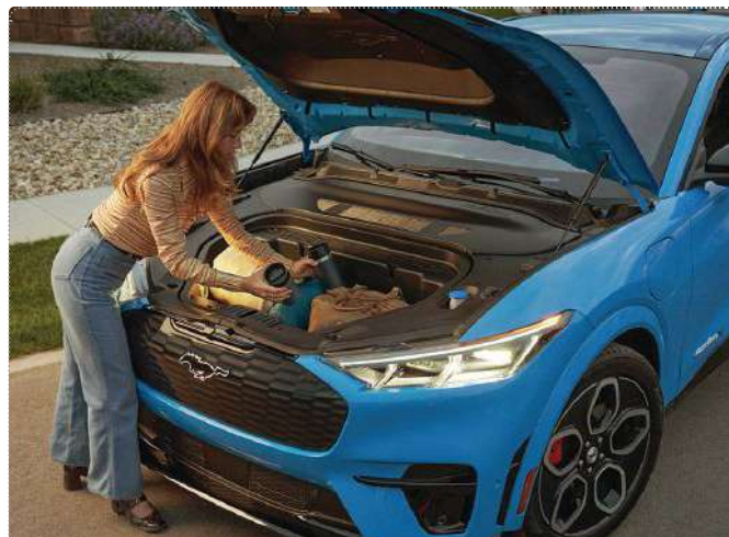
Because electric vehicles don't have engines under their hoods, many OEMs are making use of that space for front trunks, or "frunks," such as this Ford Mustang Mach-E. Its frunk is molded, in part, with recycled yogurt cups. Source: Ford Motor Co.
