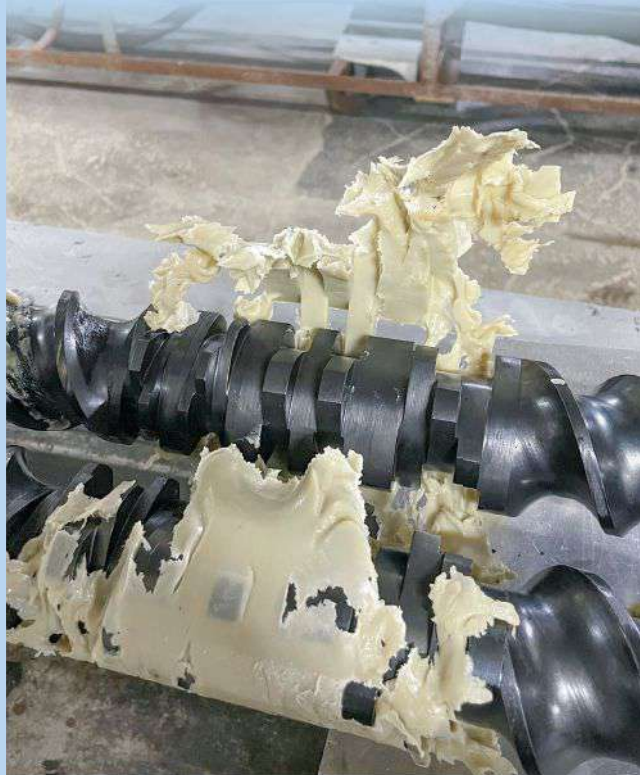
If contamination issues are severe enough to necessitate a screw pull, use a specialty purge compound designed to easily peel material off the screw. Source: Asahi Kasei North America
