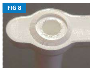
Chamfered edge around a sucker pin bore hole.
