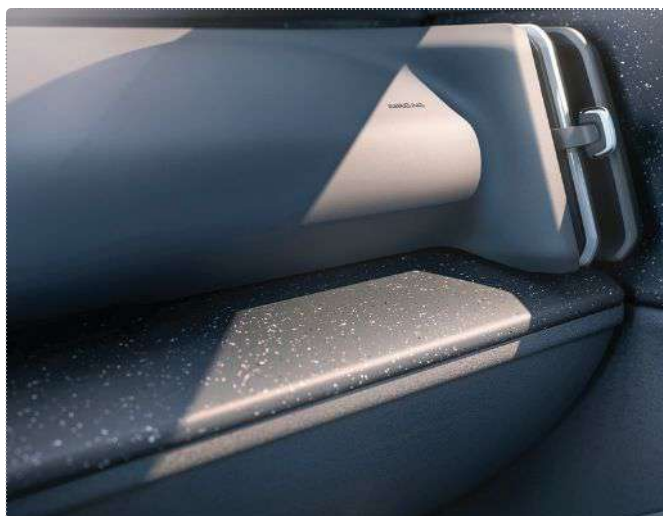
The Volvo EV30 small-electric SUV is claimed by the company to be the most sustainable vehicle it has built. Materials for molding interior trim include recycled window frames. Source: Volvo
