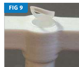
Flake formed from an aggressive undercut.
