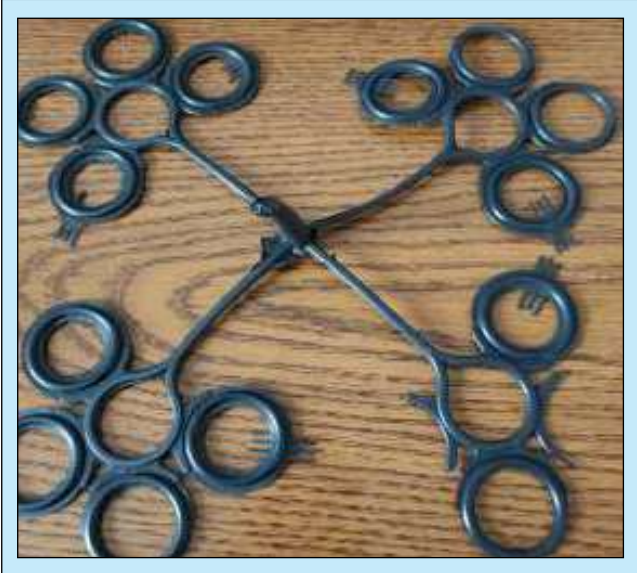
Figure 7 - parts made from a 16-cavity symmetrical o-ring mold
