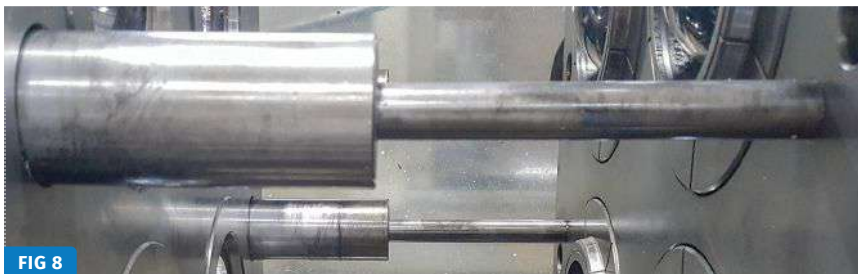
Range bolt mounted in a telescoping cylinder. Photo Credit: Jim Fattori
