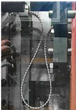
Timing belts used for pulling mold plates. Photo Credit: Jim Fattori
