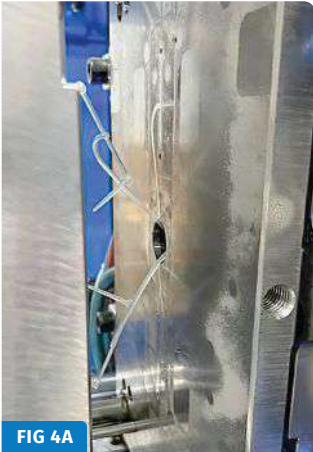
A thin runner being retained by the molding machine's nozzle tip. Photo: Westfall Technik
