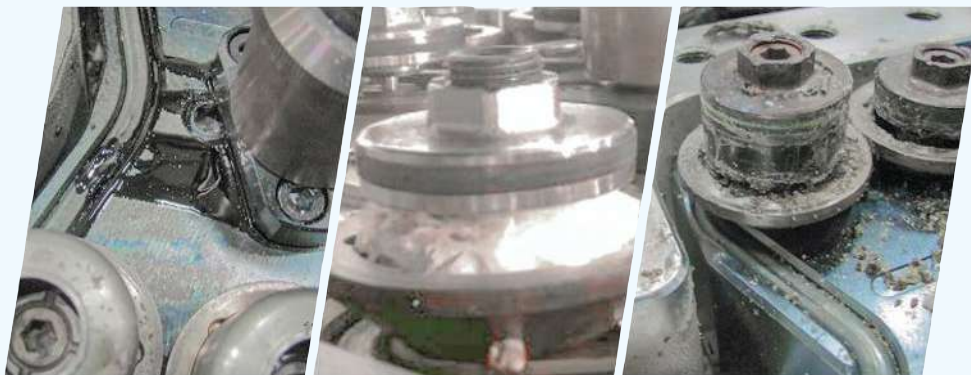
Weepage and leakage can pose issues in bioresin molding applications.
