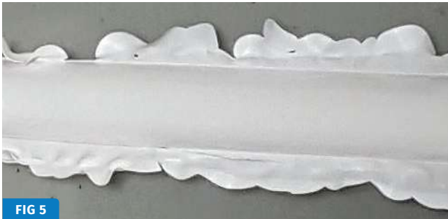
Flash traps on runners (left, before; right, after) prolong the life of a mold. Photo Credit: Jim Fattori
