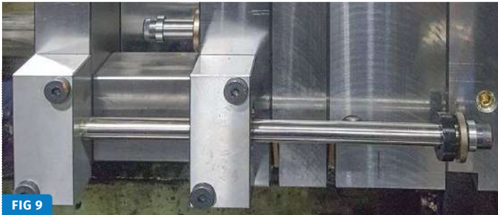
Range bolt mounted in a telescoping cylinder. Photo Credit: Jim Fattori
