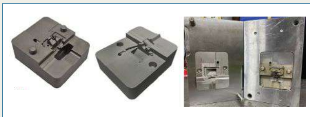
Nicolet Plastics used Mantle's metal 3D printing technology to print three complex inserts, requiring only a few hours of user interaction. Nicolet could remove all sinker EDM work required, decreasing lead time from 6 weeks to 2 weeks. Plus, the printed insert only needed 10 hours of hands-on moldmaking time. Image courtesy of Nicolet Plastics.
