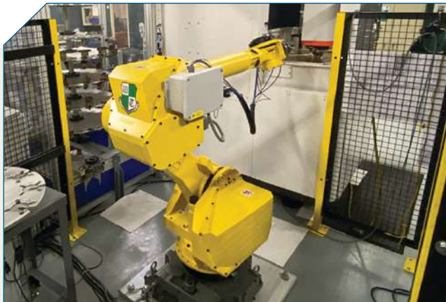
Westminster Tool, a precision toolmaker located in Plainfield, Connecticut, palletized its sinker EDM electrodes and integrated robotics to swap the electrodes during burning, allowing the EDM cell to run lights out with minimal user interaction. Image courtesy of Westminster Tool.
