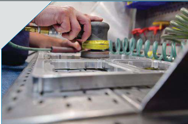
Production thermoforming mold being polished. Image courtesy of Plastic Ingenuity.
