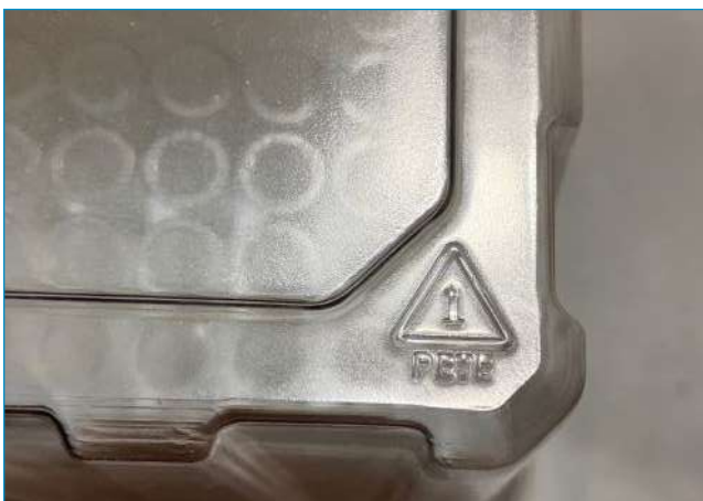
#1 Resin ID Code for PET found at the top corner of the cover. Image courtesy of Beckman Coulter.
