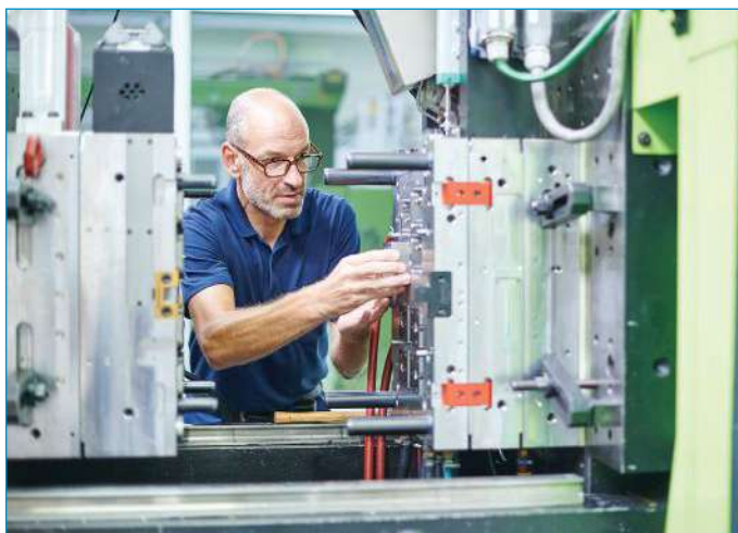
The Boucherie team carefully assembles cavities and cores into the frame and meticulously checks mold actions before putting the mold into the press for a test run.
