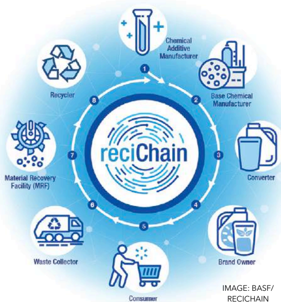
Left: This schematic shows how the reciChain blockchain-based system aims to track and validate recycled materials
