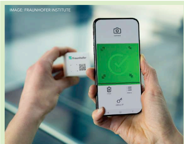
Above: Fraunhofer's SmartID system uses barcodes that capture unique surface characteristics
