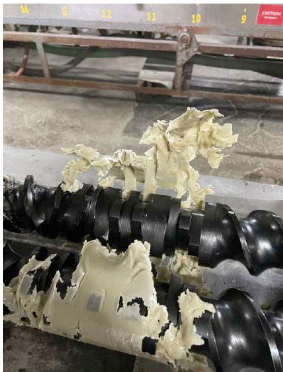
Left: Asaclean purging compound being peeled away from the screws
