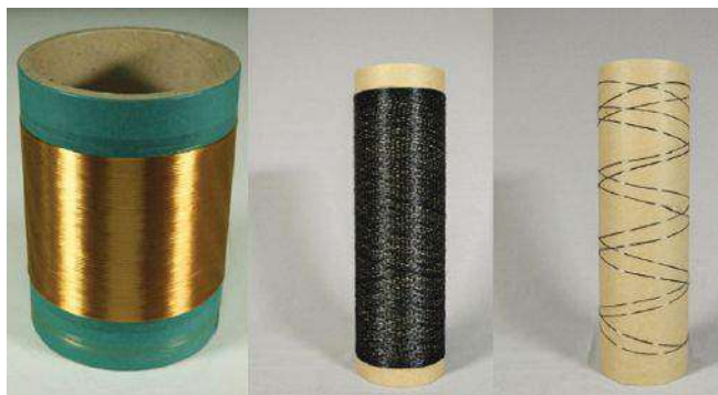
■ (Left to right) Water-spun lignin precursor fibers, stabilized lignin precursor and carbonized continuous filaments
