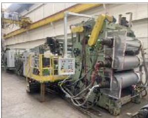
1150mm wide Omam 5 roll polishing stack
