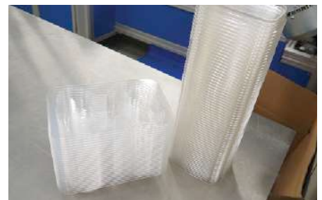
Bottom: Stacked packaging, coated with anti-block
