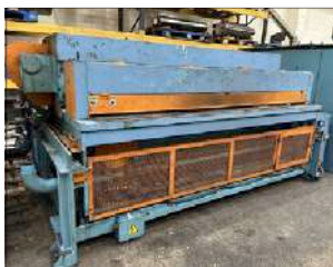
2600mm wide Caimi cross cut saw guillotine combination unit
