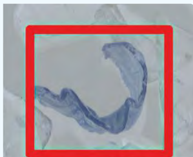
Examples of discoloration in flakes detected by optical technology.
