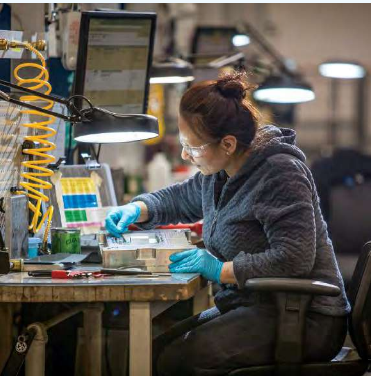
Custom mold finishing helps bring cosmetic enhancements to molded parts.
