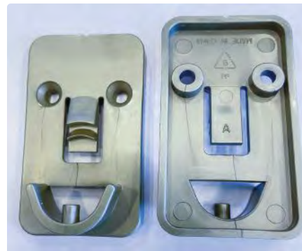
Understanding flow-front behavior can help molders address a variety of surface defects, such as weld lines. (Photo: Tony Deligio)
