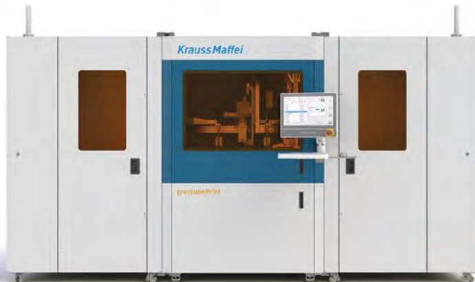
KraussMaffei's precisionPrint system features a resolution of 18-80 \mu\text{m} with a build volume of 250 × 250 × 400 mm (10 × 10 × 16 in.). (Photos: KraussMaffei)
