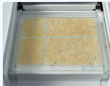
Detected contamination is highlighted in color. Pellets that are selected on the monitor are visualized on the sample tray by crosshairs.
