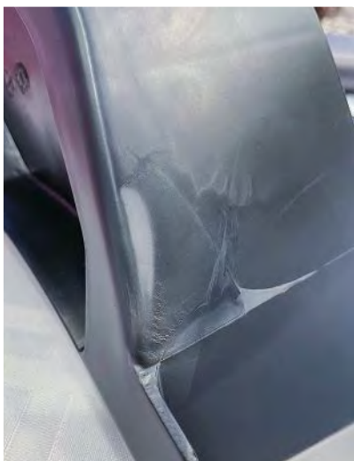
Jetting and splay in a molded part could be alleviated by investigating how the material flow front moves through the part. (Photo: Garrett McKenzie)
