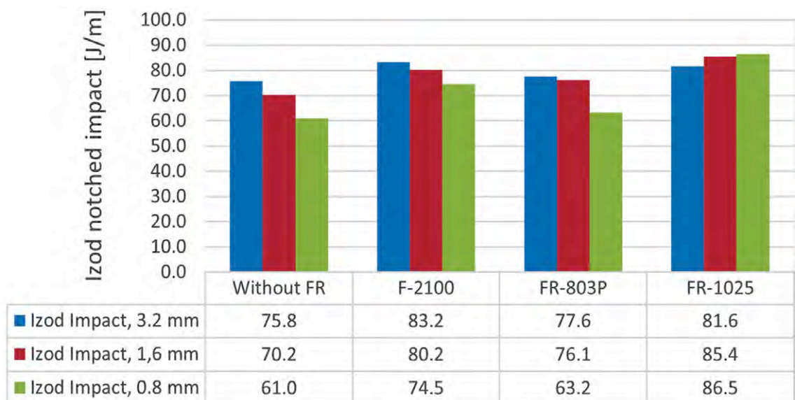
Figure 6: Impact strength as a function of sample thickness in 30% glass fibre-reinforced PBT compounds containing different brominated flame retardants
