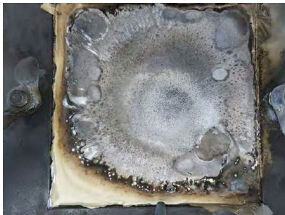
Above and below: Test set up and test plaque for a PP-compound containing 12.5 wt% glass fibre and 65 wt% Actilox HTB PP exposed for 20 minutes to a torch flame test (propane/butane-burner, 1650 W). The test specimen stayed intact (no burn-through) with a closed surface and high structural stability
