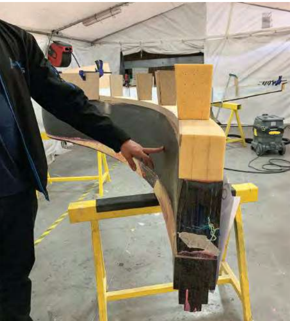
FIG. 2 Stock manufacturing using pre-cured plates
