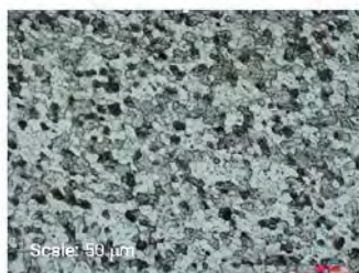
As-deposited Melded Al2139
