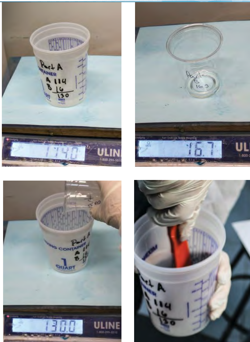
FIG. 2 Weighing, mixing a two-part resin system
