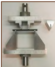
Three & Four Point Flexure Test Fixture ASTM D 790, D 6272, D 7264
