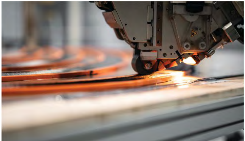
FIG. 2 Stock manufacturing using pre-cured plates
