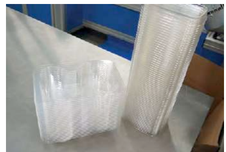
Bottom: Stacked packaging, coated with anti-block
