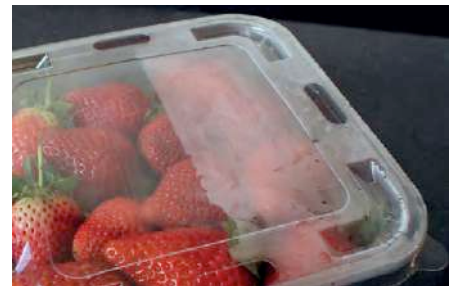
Top: Partly coated with anti-fog
