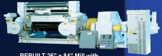
REBUILT 26" x 84" Mill with Motorized Roll Nip Adjustments
