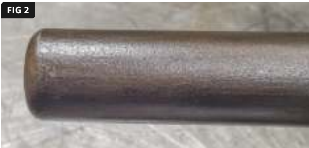
FIG 2 A rusted leader pin with a high COF. Photo Credit: J. Fattori
