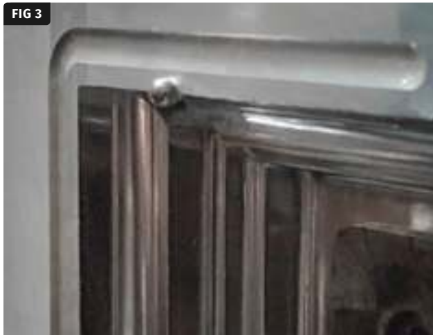
FIG 3 Mold damage from ball bearings. Photo Credit: J. Fattori
