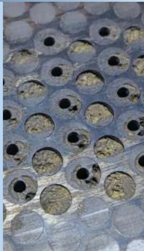
FIG 1 Acid attack has caused serious damage on the cutting face of this pelletizer. Photo Credits: Maag Group
