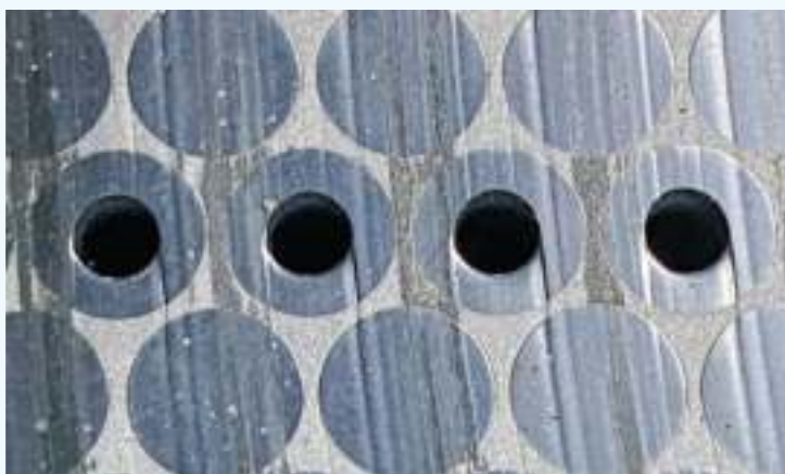
FIG 3 Cutting face showing accelerated wear due to local chemical attack, which has reduced the sharpness at the edges of the extrusion holes.
