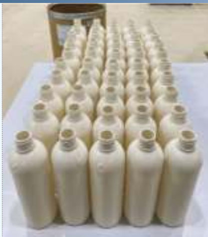
Cure time before packaging may be required for PHA/PLA blow molded bottles.
