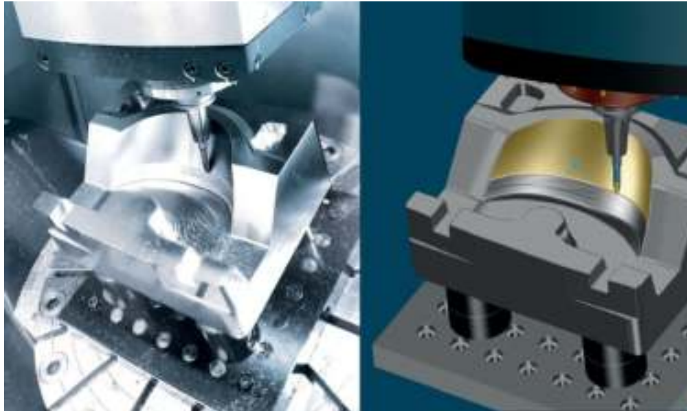
Mold builders can automate the general mold design by using CAD/CAM to develop a template.
