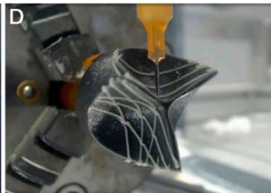
Custom 3D-printed heart valve
