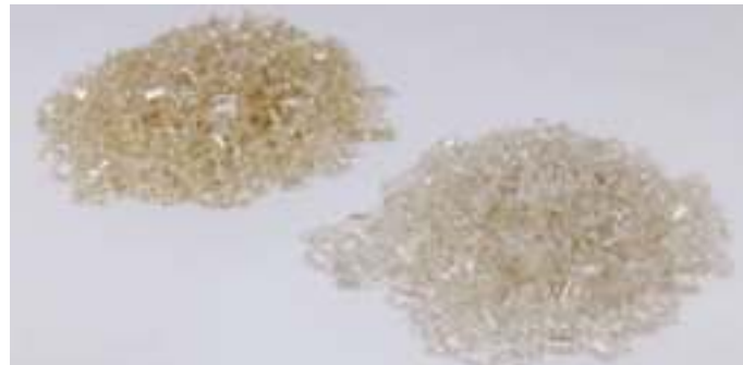
Left side: PET after 4 passes (without rBOOST) Right side: PET after 4 passes with rBOOST
