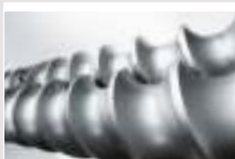
STS Mc11 - the next generation of Coperion's STS twin screw extruders. Featuring a specific torque of 11.3 Nm/cm 2 .
