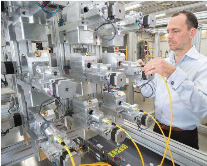
FIG. 4 Laser CVD, scaling short SiC fiber production
