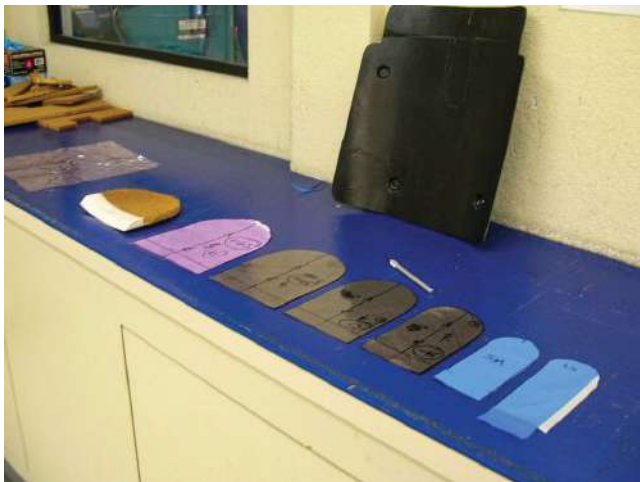
FIG. 3 Repair material preparation
