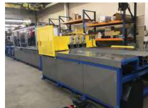
In line Cut-Off Saw Systems travels and cuts product at line speed
