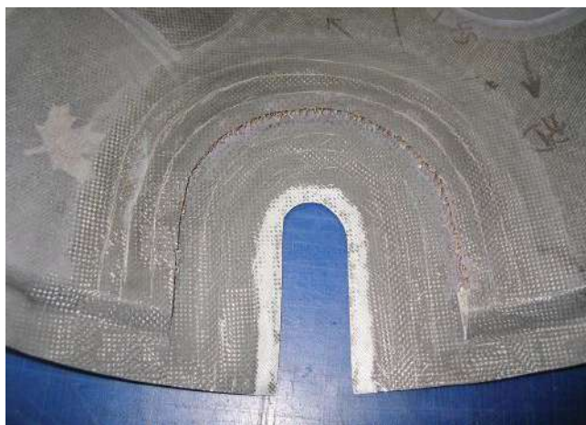
FIG. 2 Machining the inner skin, core
