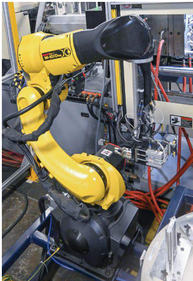
A six-axis Fanuc robot removes parts and adds inserts in an automated production cell.
