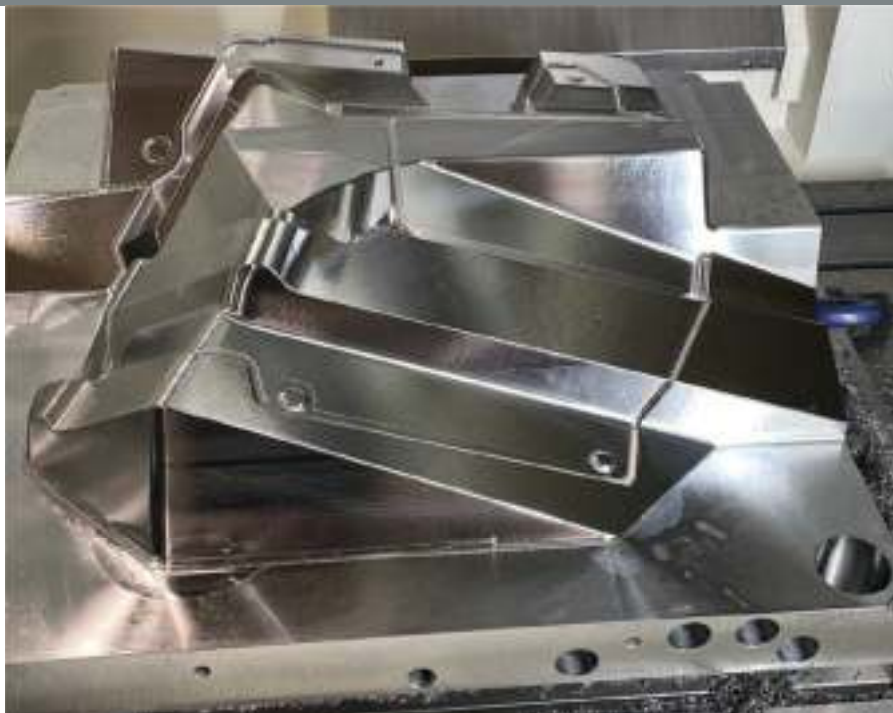
Machining Technology was able to reduce polishing and eliminate EDM burning when machining cavities using hyperMILL 3D strategies.
