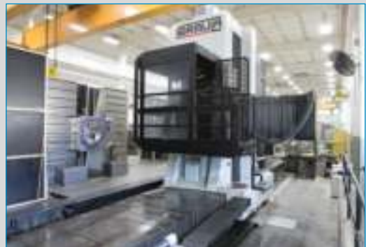
The OMV Formula five-axis high-speed mill, with its automatic head changing, large-capacity toolchanger, laser tool setting and on-machine probing, is well suited for unattended machining on medium to large blocks.
