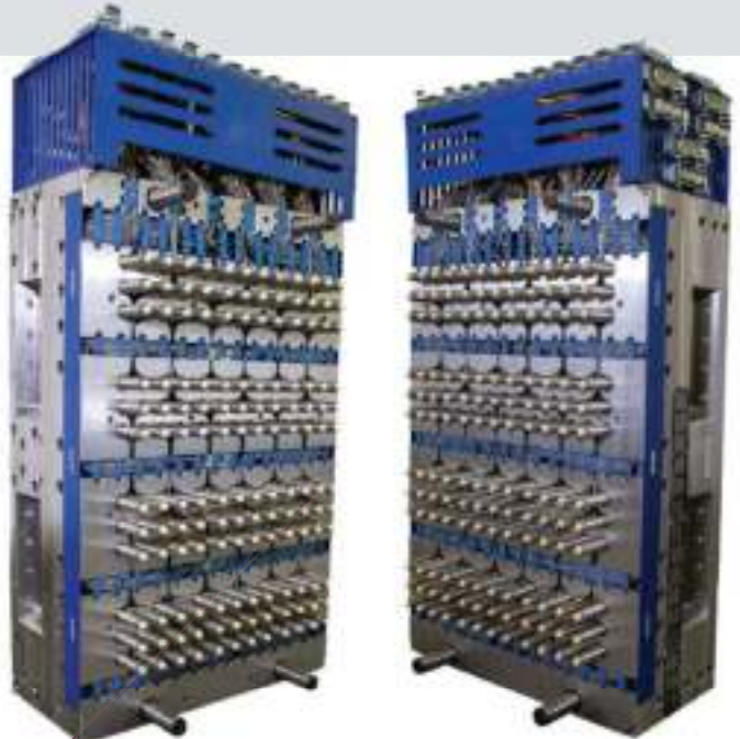
This 144-drop hot half shows very closely positioned nozzles. Nozzle size and spacing are among the critical factors that help determine the size and cost of the hot runner system, mold and molding machine required for optimum production of a given part.
