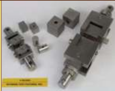
SHOWN RIGHT: ASTM C297 SANDWICH PANEL FLATWISE TENSILE TEST FIXTURE MODEL: WTF-FT 2" BLOCKS
