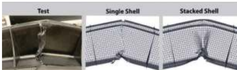
FIG. 3 Comparison of force-displacement curves and failure behavior between test and simulation
