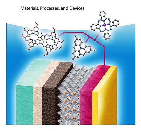
The use of perovskite-structured materials to produce high-efficiency solar cells is a subject of growing interest for academic researchers and industry professionals alike. Due to their excellent light absorption, longevity, and charge-carrier properties, perovskite solar cells show great promise as a low-cost, industry-scalable alternative to conventional photovoltaic cells.
