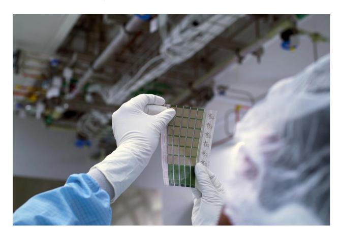
MIT engineers have developed ultralight fabric solar cells that can quickly and easily turn any surface into a power source.
