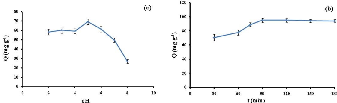
**Fig. 4.** Adsorption capacity of MMIP at different pH containing the  $3 \text{ mmol L}^{-1}$  4-NP in a buffer ranging from 2 to 8 (a), kinetic adsorption curves for 4-NP containing the  $5 \text{ mmol L}^{-1}$  4-NP (b).
