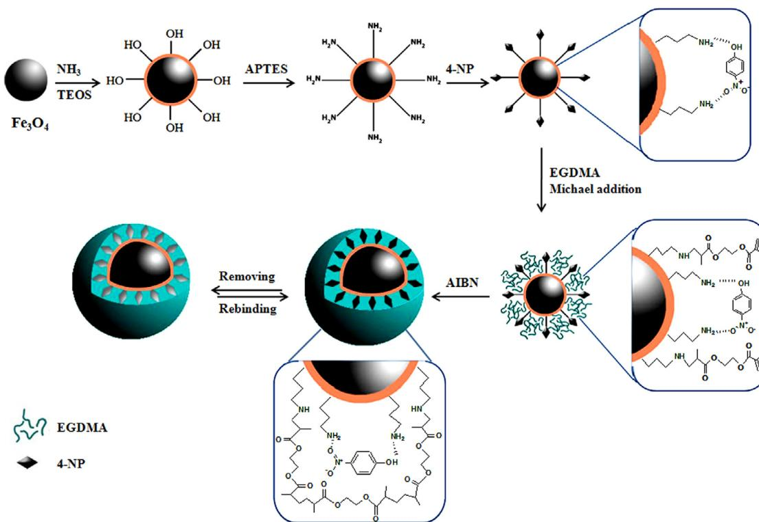
**Fig. 1.** Scheme of the synthetic route for 4NP-MMIP by surface immobilized template strategy.
