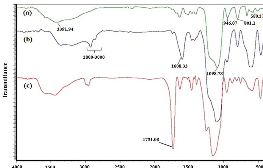
**Fig. 2.** FT-IR spectra of  $\text{Fe}_3\text{O}_4@\text{SiO}_2$  (a),  $\text{Fe}_3\text{O}_4@\text{NH}_2$  (b) and  $\text{Fe}_3\text{O}_4@\text{MIP}$  (c).
