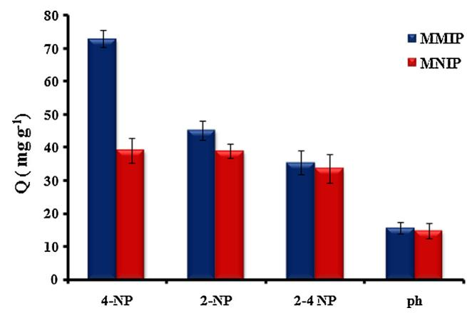
Fig. 6. Adsorption selectivity for 4-NP and analogous compounds by MMIP and MNIP under optimized conditions.
