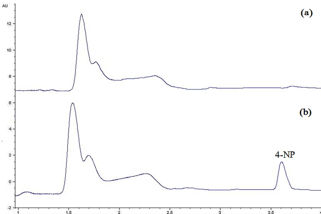
Fig. 7. The chromatograms of extracted 4-NP from Persian Gulf (a) and spiked sample with 100 µg L<sup>-1</sup> of 4-NP (b) by MMIP.
