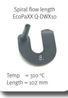
EcoPaXX has wide processing window which makes it easy to process and suitable for large mass production. EcoPaXX enables superb "bonding" performance in over-mold design. Compared to PPAs, EcoPaXX superb flow and slow crystallization speed enables excellent surface quality even up to 60% GF reinforcements. Superb flow means better over-mold stability/bonding, less internal stress, more design freedom for faucet system manufacturers.
