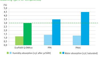
EcoPaXX absorbs 30% less moisture than other polyamide based materials in combination with excellent hydrolitic and dimensional stability. Thanks to its long aliphatic chains EcoPaXX offers superior chemical resistance, which is especially important when in contact with chlorinated water. It has passed more than 1 million lifetime cycles testing in varying water temperatures.
