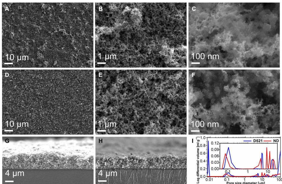
**Fig. 3. Surface morphologies and pore distributions of MEAs with conventional D521 ionomer and ND ionomer.** SEM results of (A to C and G) MEA with conventional D521 ionomer and (D to F and H) MEA with ND ionomer. (I) MIP results of MEA with conventional D521 ionomer (blue) and ND ionomer (red). The inset is an enlarged graph showing the pore distribution near 0.1 to 10  $\mu\text{m}$ .
