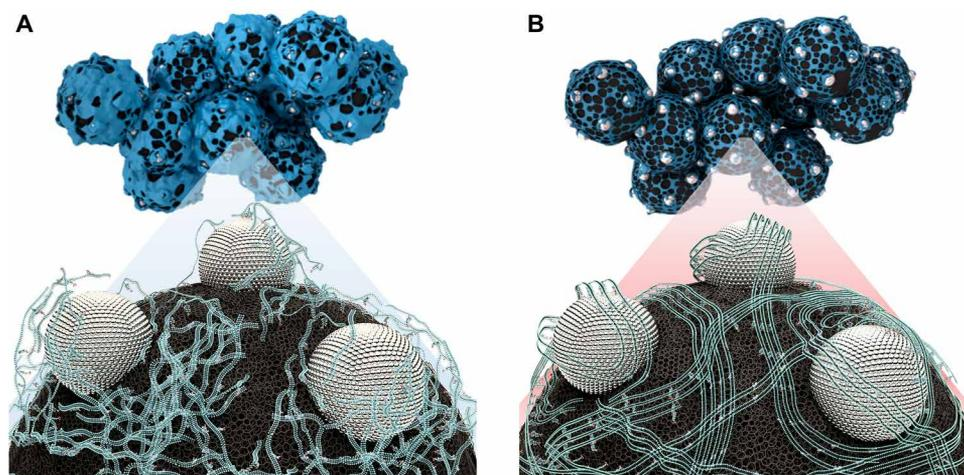
**Fig. 1. Schematics of Nafion ionomers on the catalyst surfaces.** (A) Distribution of conventional ionomers synthesized by emulsion polymerization. (B) Distribution of the laboratory-made ionomers synthesized by SCF process. Enlarged conceptual diagram showing the distribution of both conventional and prepared ionomer on the Pt/C catalyst surface. The SCF process contributes to the formation of nanodispersed Nafion ionomer, leading to improved electrochemical performance and durability.
