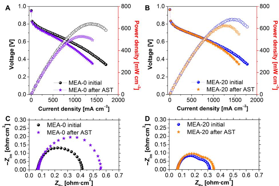
**Fig. 4. Polarization curves and EIS results of MEAs with conventional D521 ionomer and ND ionomer before and after AST.** Fuel cell performances of MEAs before and after AST. (A) MEA with conventional D521 ionomer. (B) MEA with ND ionomer in air. EIS results for MEAs before and after AST. (C) MEA with conventional D521 ionomer. (D) MEA with ND ionomer in air.
