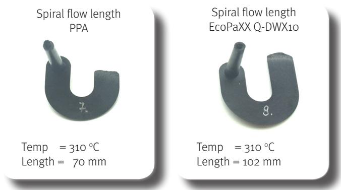
EcoPaXX has wide processing window which makes it easy to process and suitable for large mass production. EcoPaXX enables superb “bonding” performance in over-mold design. Compared to PPAs, EcoPaXX superb flow and slow crystallization speed enables excellent surface quality even up to 60% GF reinforcements. Superb flow means better over-mold stability/bonding, less internal stress, more design freedom for faucet system manufacturers.
