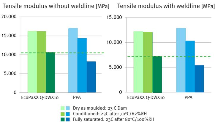
EcoPaXX Q-DWX10 exhibits a 30% higher tensile modulus vs. PPAs, even when fully saturated in water. This is confirmed by customers, who see an extremely low decrease in torque strength of faucet mixing valves made from EcoPaXX after long-term 90°C water contact. High tensile modulus even at the weldline, allows design of complex parts.
