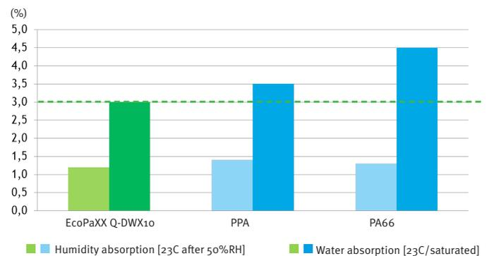
EcoPaXX absorbs 30% less moisture than other polyamide based materials in combination with excellent hydrolytic and dimensional stability. Thanks to its long aliphatic chains EcoPaXX offers superior chemical resistance, which is especially important when in contact with chlorinated water. It has passed more than 1 million lifetime cycles testing in varying water temperatures.
