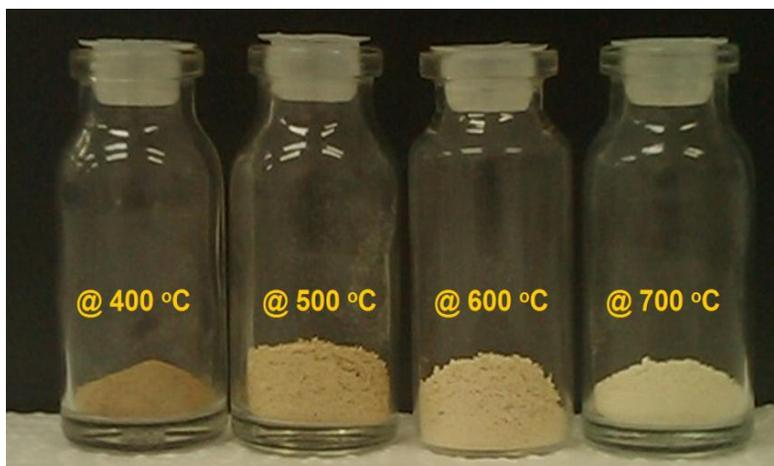
**Fig. 1. Lab photograph of prepared ZnO-NPs at different calcination temperatures.**
